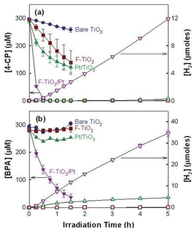
Figure 4. The degradation of the substrates 4-CP in chart A and BPA in chart B and the creation of hydrogen as water splits (Kim & Choi, 2010).
